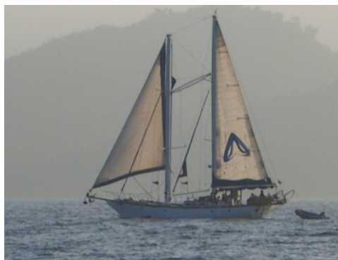
Note above the roller-furling foresail with wishbone boom on this staysail Schooner.
