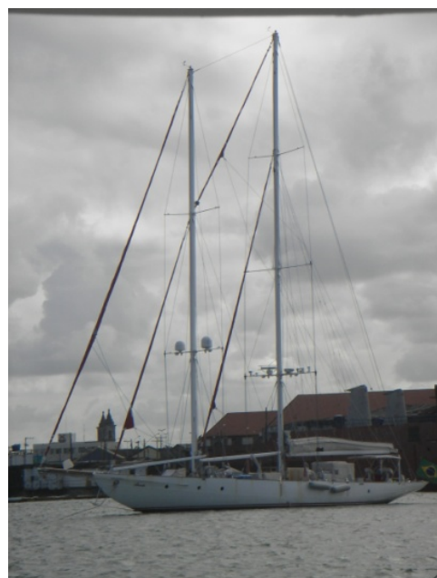
Staysail Schooner at anchor in Recife (above). Note roller furling upper staysail.
